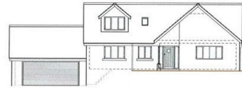
Front (East) Elevation
