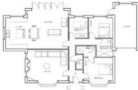
GROUND FLOOR PLAN PLOT 4 BUNGALOW 3 BED DETACHED BUNGALOW 1 FLOOR TOTAL = 123sqm / 1324sqft PLUS GARAGE = 18sqm / 194sqft
