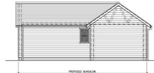
PROPOSED SIDE ELEVATION SCALE 1:50
