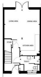
Ground Floor Plan Layout Scale 1:100
