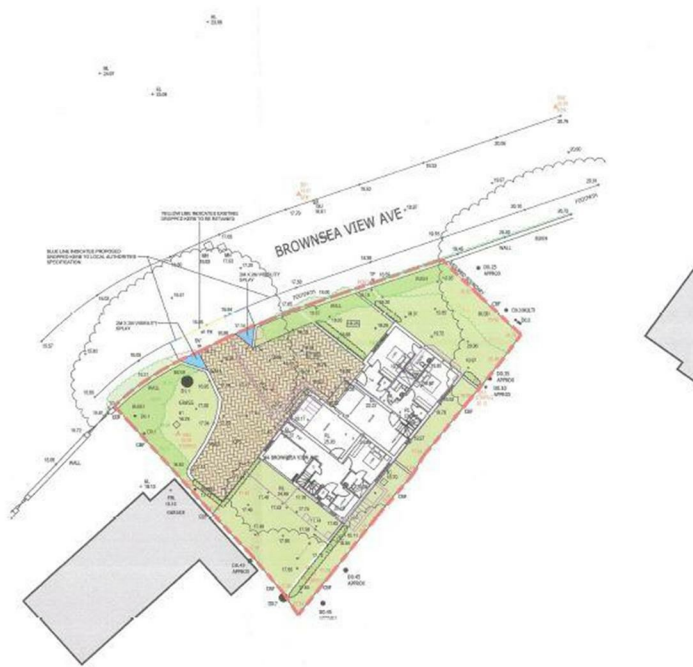
SITE PLAN: BASED ON TOPOGRAPHICAL SURVEY INFORMATION SCALE 1:200
