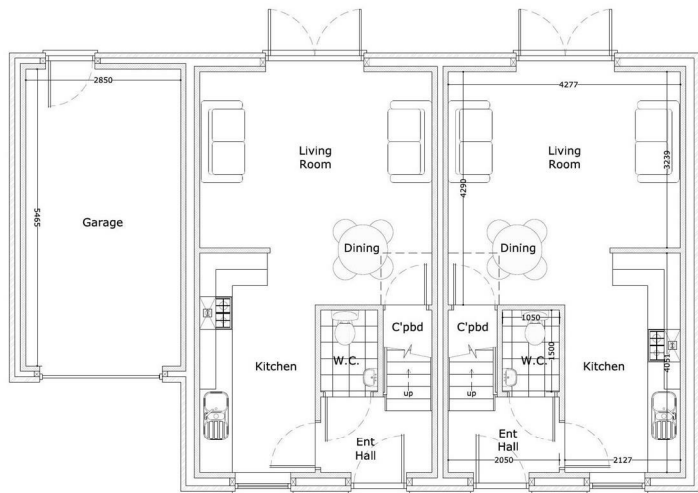
Proposed Ground Floor Plans Gross Floor Area = 78m 2 or 839ft 2 (Exc. Garage) Gross Floor Area = 63m 2 or 678ft 2 (No Garage Type) Garage Gross Floor Area = 15.5m 2 or 166ft 2
