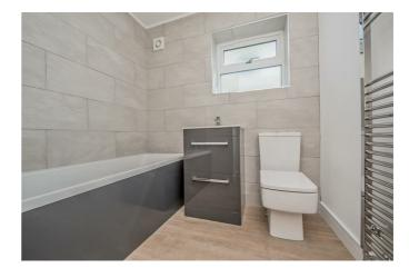
Double glazed window, a modern white suite comprising of a panelled bath with a plumbed shower above and a glazed side screen, wash basin set into a vanity unit, low flush WC, modern tiling, extractor fan, inset ceiling lights
