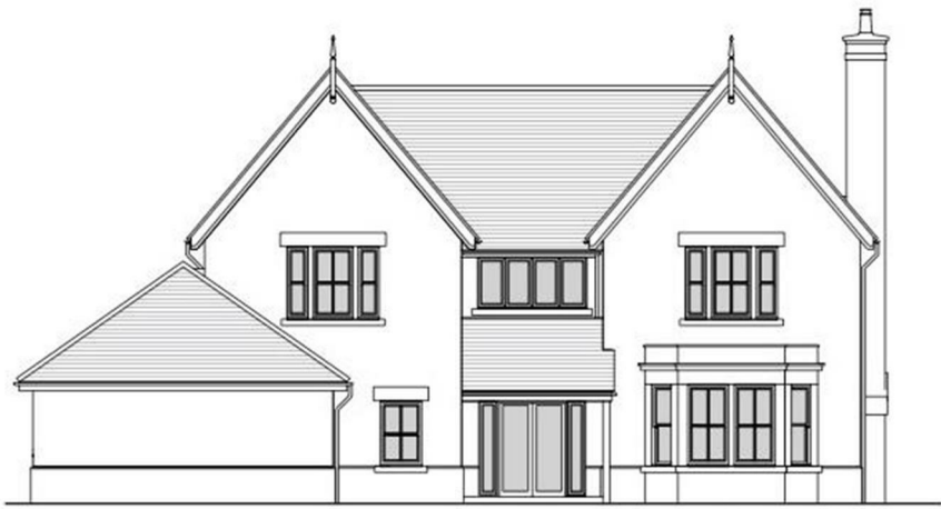
NORTH ELEVATION AS PROPOSED
