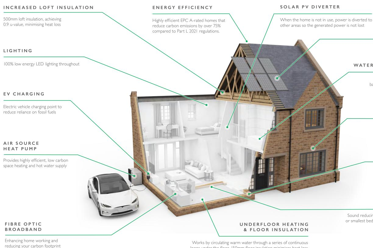
Works by circulating warm water through a series of continuous loops under the floor. I50mm floor insulation minimises heat loss
