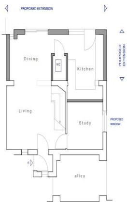
Proposed Ground Floor Plan at 1:100 scale
