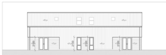
Proposed East Elevation 1:100
