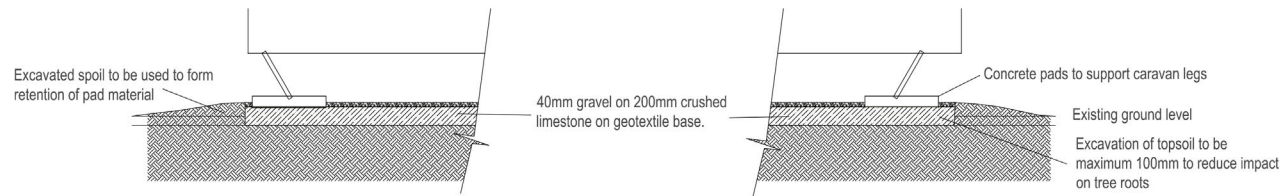
CROSS SECTION OF PROPOSED PADS FOR CARAVANS 1 : 50
