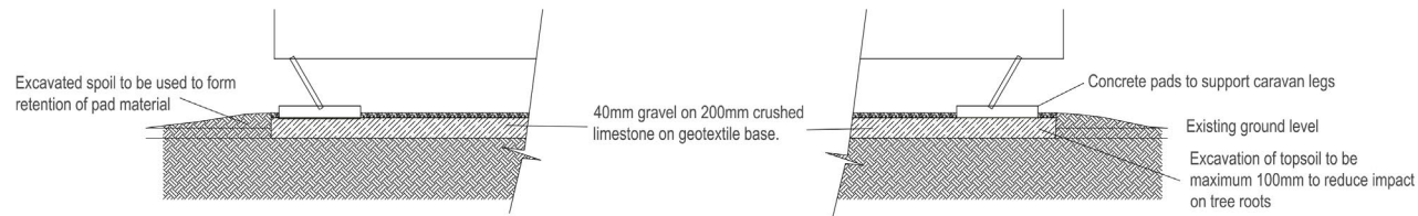
CROSS SECTION OF PROPOSED PADS FOR CARAVANS 1 : 50
