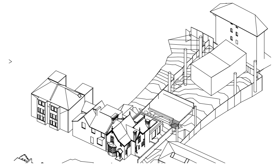
Manipulated the roof scope over two floors to take in consideration that we didn't want the building to be too high so decided on a shallow butterfly roof with the higher pitch towards the north of the boundary
