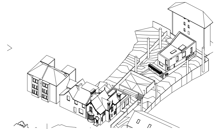
Articulated the elevations – positioning windows so that direct overlooking is reduced. The building
