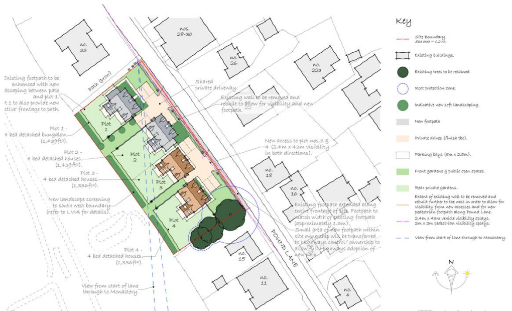
SITE LAYOUT PLAN AS PROPOSED 1:200
