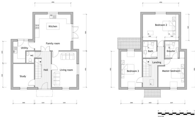
GROUND FLOOR LAYOUT PLAN 1:50 NEW HOUSE PLOT 2
