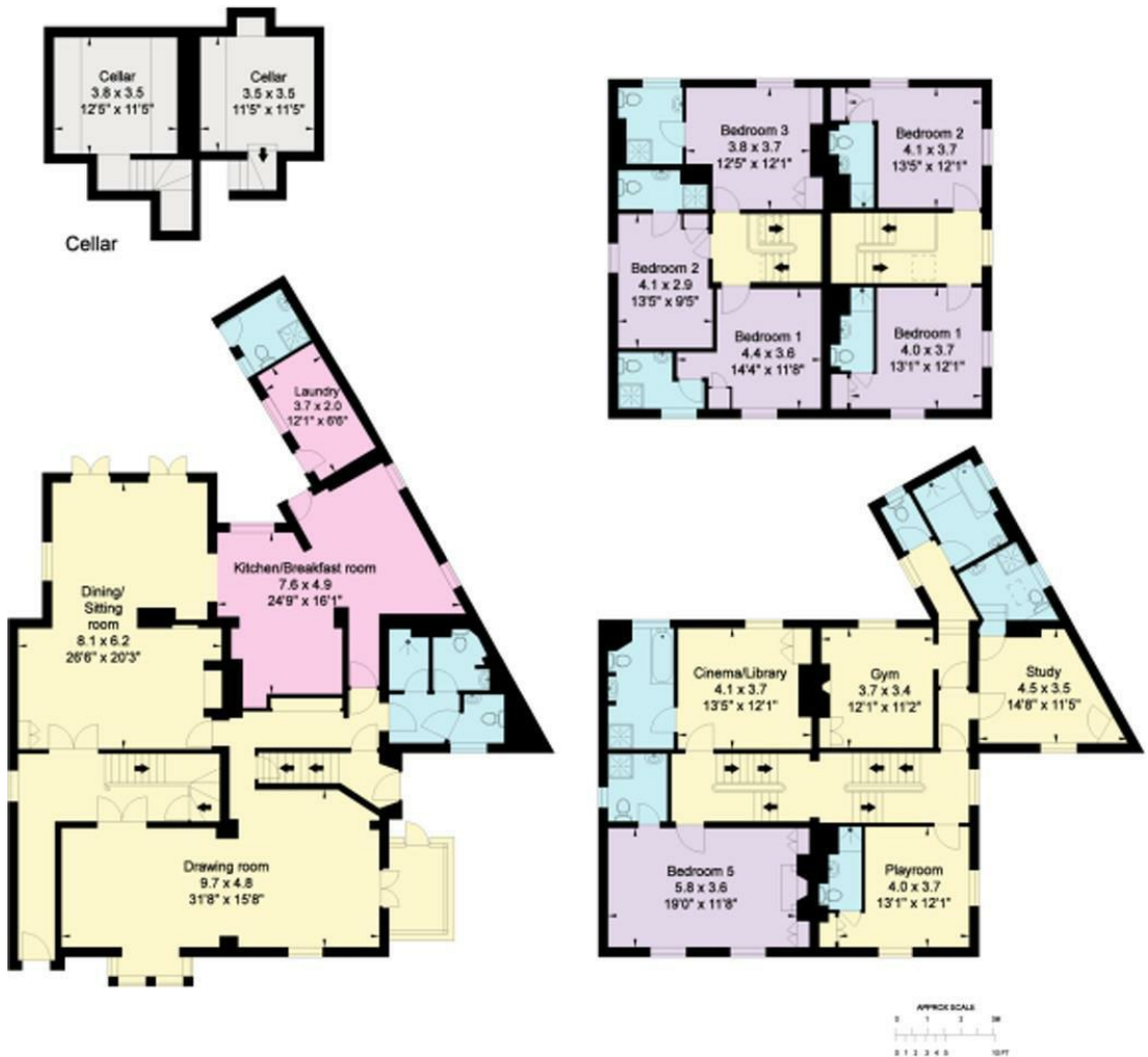
Arden House Stratford upon Avon (Proposed option for use as one dwelling)
