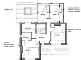
First Floor Plan Proposed 1: 100
