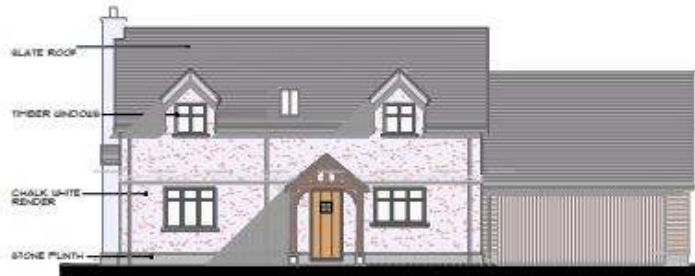
FRONT (SOUTH EAST) ELEVATION
