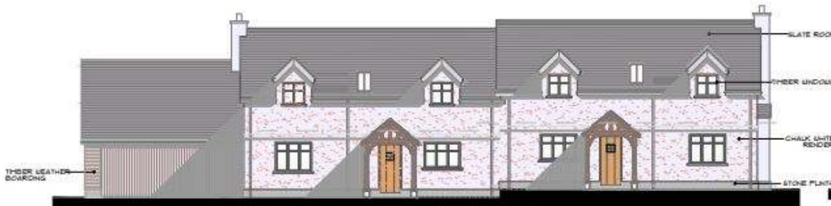
FRONT (SOUTH EAST) ELEVATION
