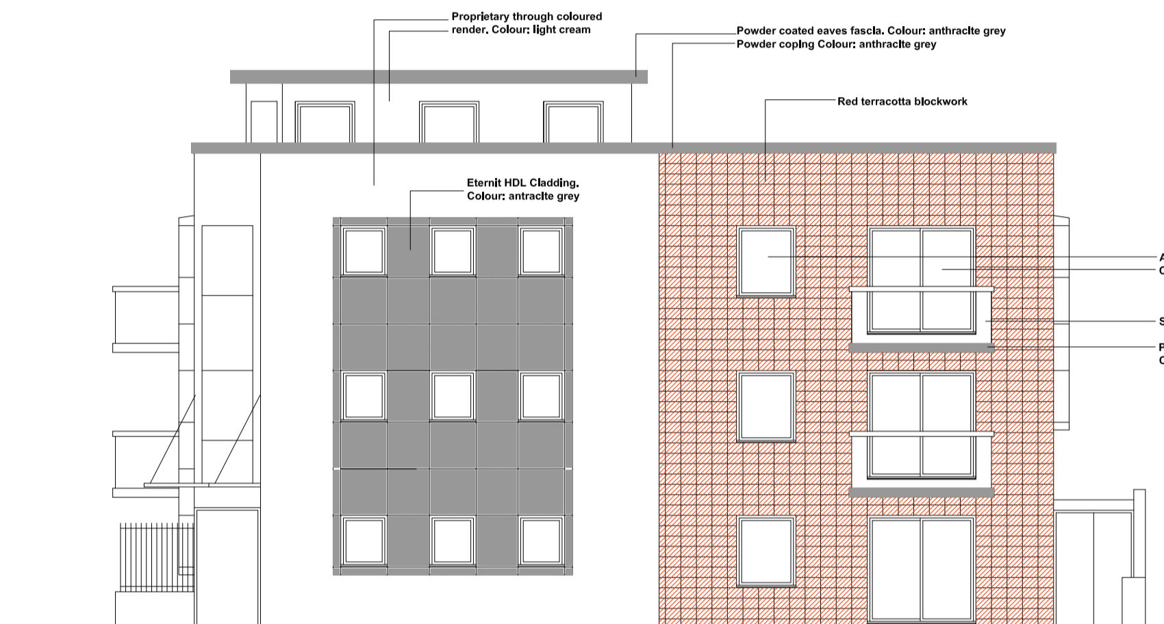
EXISTING SOUTH ELEVATION to Snakes Lane East 1:100
