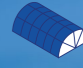
Barrel Vaulted Roof
