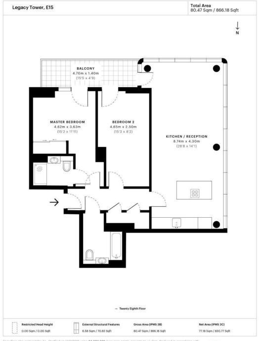
Spec floor plan captured for JLL, Stratford on 14/11/2018 using 34,804,939 laser scan points, accurate to +/- 3cm. Produced in accordance with Royal Institution of Chartered Surveyors Property Measurement Standards, incorporating International Property Measurement Standard (IPMS). If you intend to rely on any measurement in a transaction you should perform your own checks. Plot/Gardens illustrative only and excluded from all area calculations. Specific Sebe50535d583ea108e06356d
