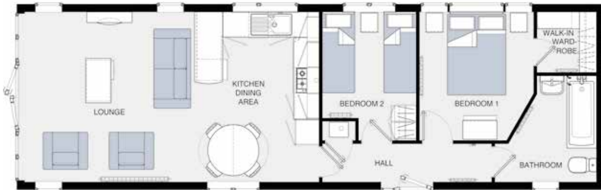
45' x 14' (13.716m x 4.267m) 2 bedrooms (master with walk-in wardrobe) and family bathroom
