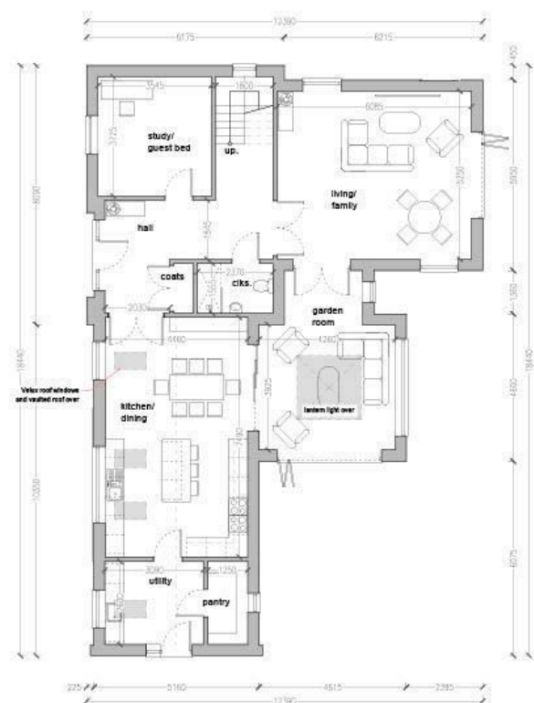
Ground floor plan Footprint area = 165m² Ground floor internal area = 144m² First floor internal area = 74m²
