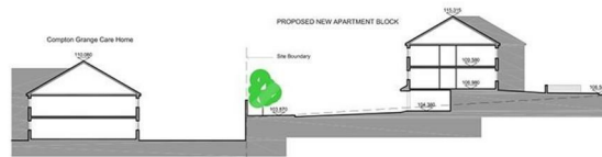
Section A-A through site Scale 1:200
