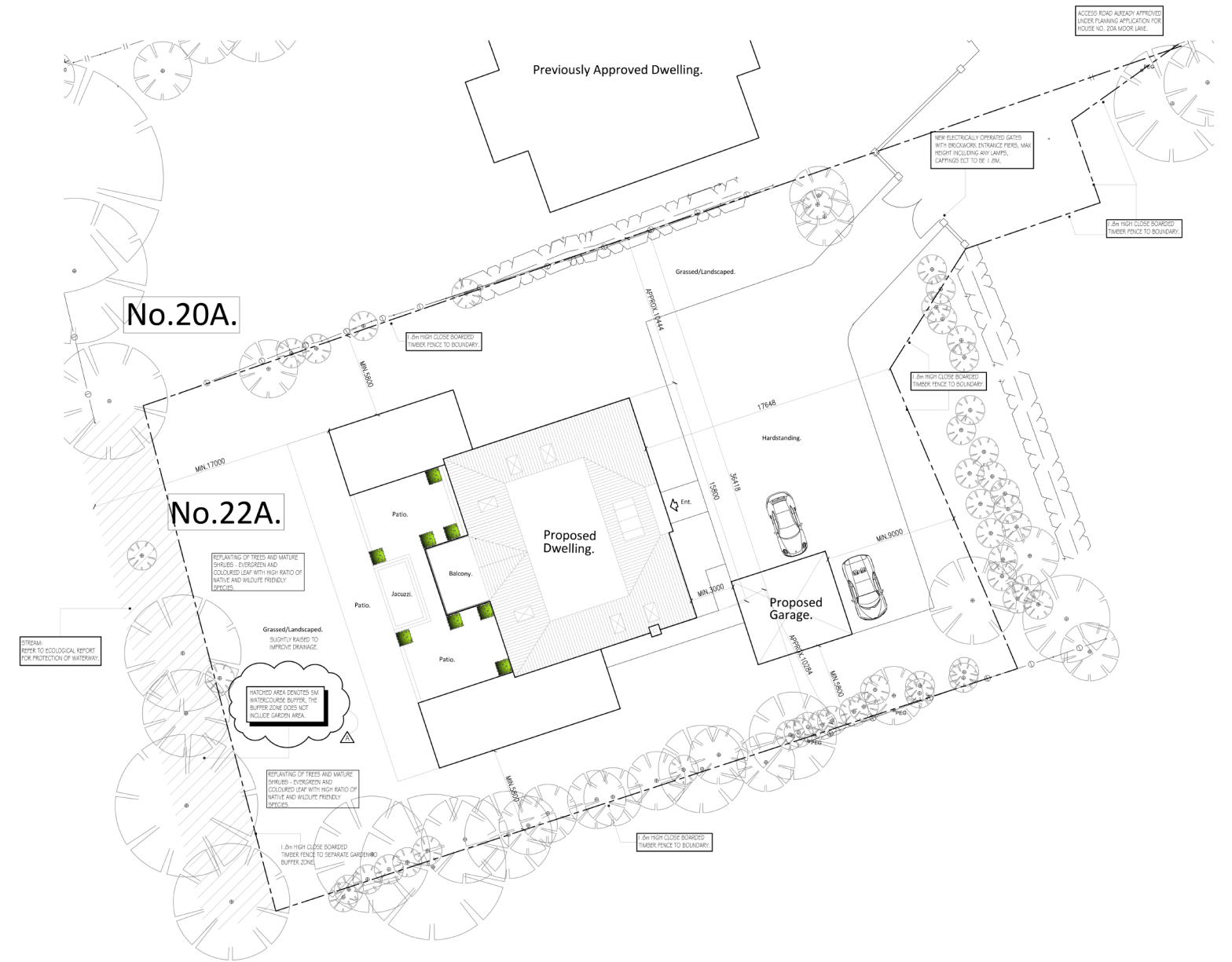
Proposed Site Layout Plan. Gross Site Area: 2215m 2 (Not including previous approved Access Road.)
