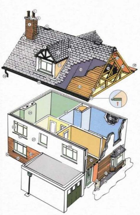
(19) Rainwater downpipe (20) Verge boards /skews (21) Soffit boards (22) Partition wall (23) Lath / plaster (24) **Chimney breast** (25) Window pointing (26) Window sills (27) Rendering Brickwork / pointing (28) (29) Bay window projection (30) Lintels (31) Cavity walls / wall ties (32) Subfloor ventilator (33) Damp proof course (34) **Base course** (35) Foundations (36) Solum (37) Floor joists (38) Floorboards 39) Water tank (40) Hot water tank
