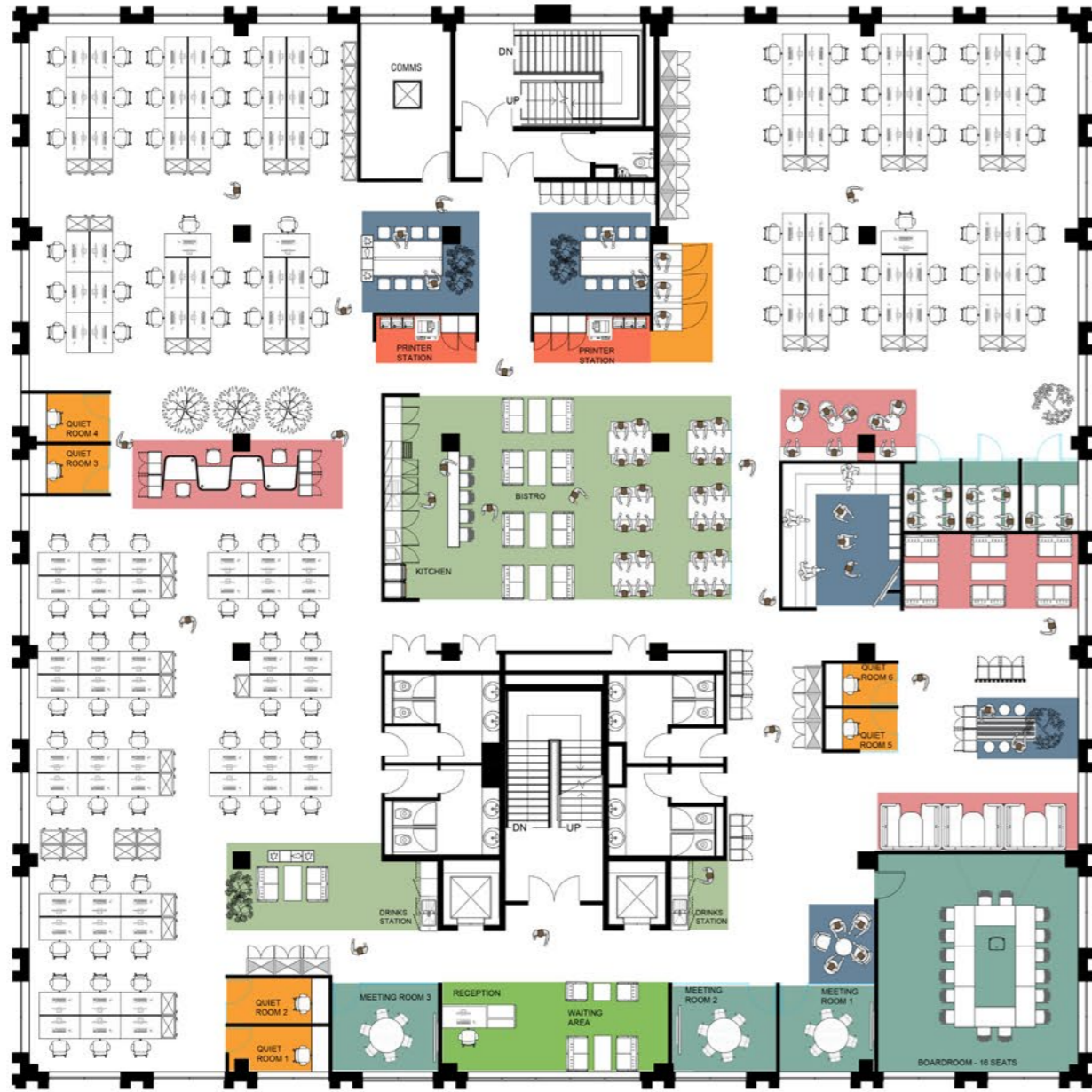
Occupational density in open plan 115 desks (1-10m 2 per person). This excludes the agile working areas.
