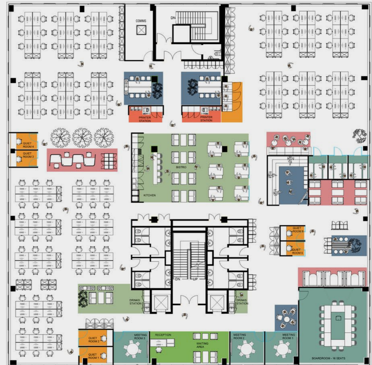
Occupational density in open plan 120 desks (1-10m 2 per person). This excludes the agile working areas.
