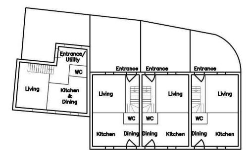
PROPOSED GROUND FLOOR PLAN SCALE 1:200
