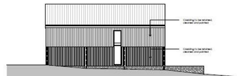
Proposed East Elevation
