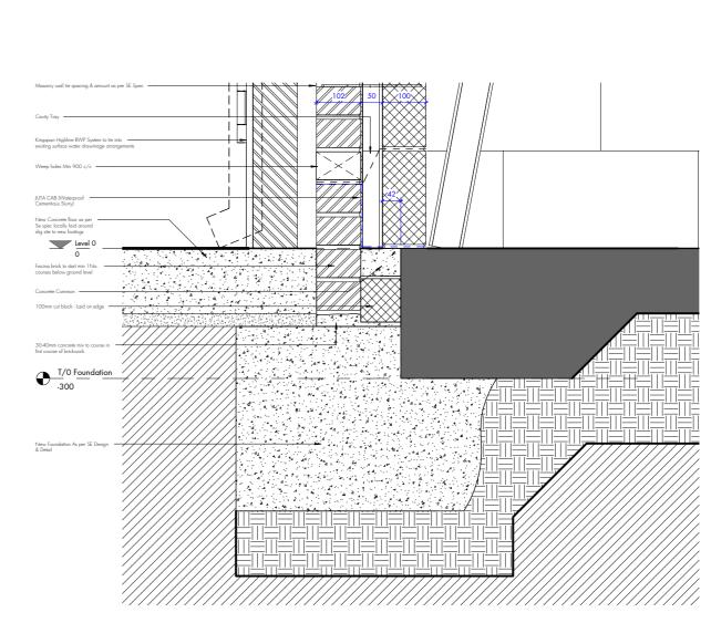
Kingspan Multibeam cladding rail system to specialsit sub-contractors design
