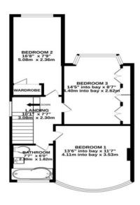
TOTAL FLOOR AREA: 1348 sq.ft. (125.3 sq.m.) approx Measurements are approximate. Not to scale. Illustrative purposes on Made with Metropix C2024
