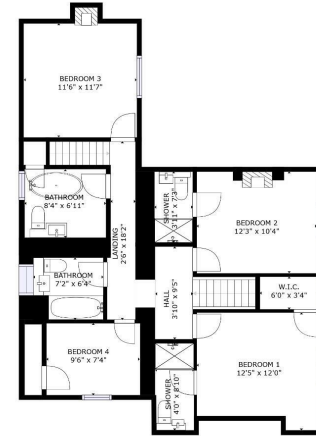
FLOOR 2 GROSS INTERNAL AREA FLOOR 1: 1312 sq. ft. FLOOR 2: 961 sq. ft. TOTAL: 2273 sq. ft. NOTE: AREA DOES NOT INCLUDE PORCHES, PATIOS, DRIVEWAYS.
