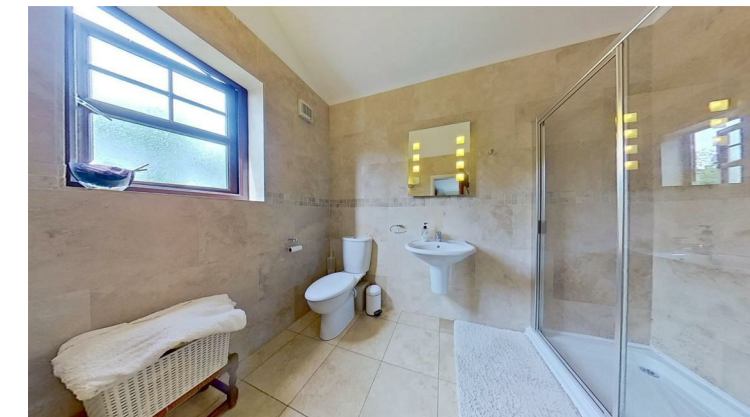
Modern white suite with chrome style fittings comprising: shower enclosure with Mira shower, glazed shower screen and glazed door; low level dual-flush WC; and wall mounted wash hand basin with mixer tap. Travertine tiled walls and travertine tiled floor, chrome ladder style towel radiator, wall light point, extractor, illuminated wall mirror, and UPVC double glazed window with obscured glass.
