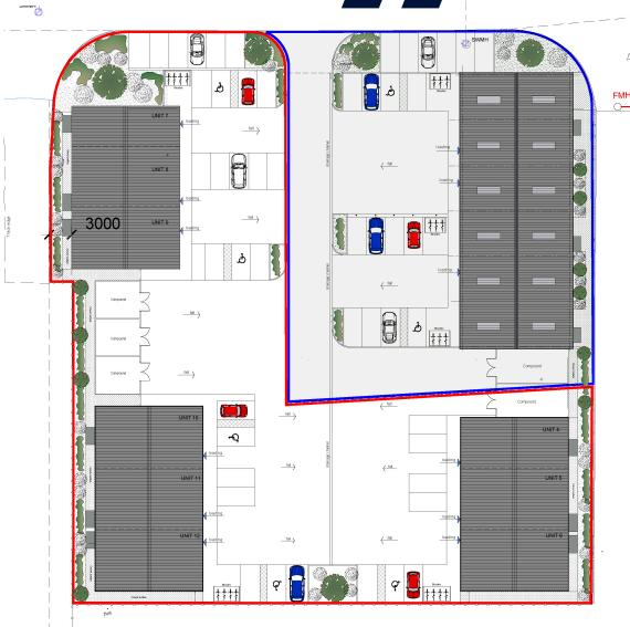
Units at Borders II Industrial Estate will comprise new build industrial/ warehouse units constructed of steel portal frame clad with plastic coated metal insulated panels beneath a roof of similar materials incorporating approximately 15% lighter panels.
