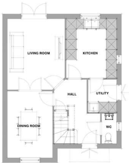
01 UNIT B: GROUND FLOOR PLAN 1:50 @ A1 / 1:100 @ A3
