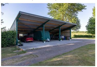
3 bay steel frame with concrete panel and concrete block walls, boarded and steel profile cladding, mono-pitched steel box profile roof, concrete floor, concrete apron with overhang, power, lights and water.
