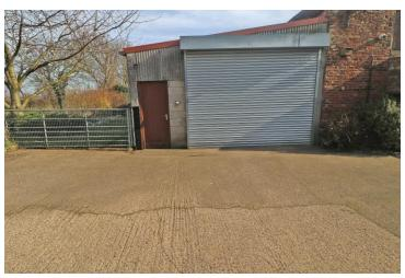
PORTAL FRAME 5 BAY CONSTRUCTION:75' 5" x 42' 7" (23,052m x 13,653m) Light and power. Electric roller at one end of the construction and roller doors to the other, Concrete floor and concrete block walls.
