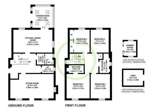
APPROXIMATE GROSS INTERNAL AREA GROUND FLOOR = 914 SQ FT / 84.9 SQ M FIRST FLOOR = 785 SQ FT / 72.9 SQ M OUTBUILDINGS = 133 SQ FT / 12.4 SQ M TOTAL = 1832 SQ FT / 170.2 SQ M
