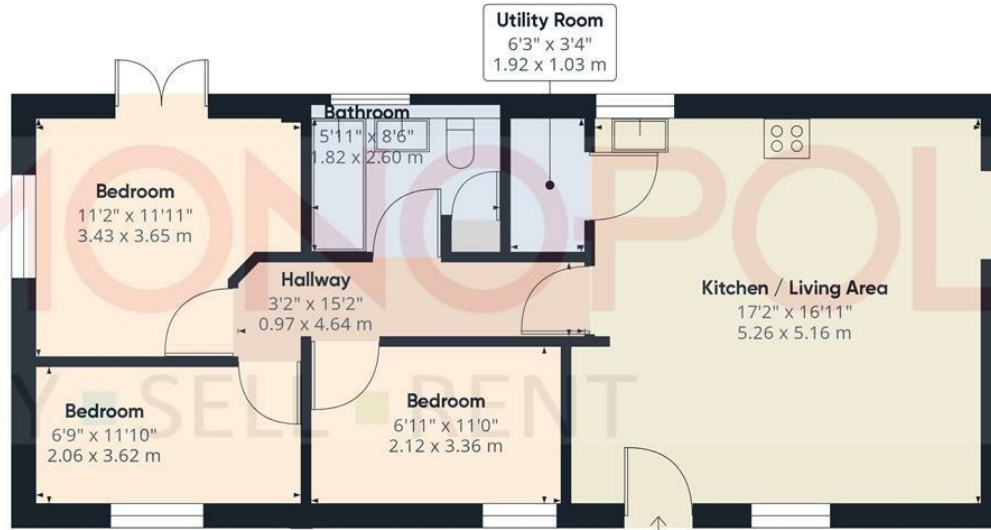
Ground Floor Building 1
