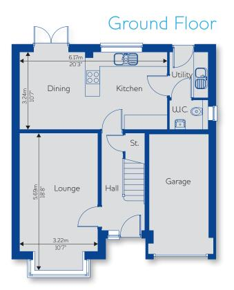
Note: All dimensions are maximum and account for alcoves, and a tolerance of  $\pm$  75mm should be allowed.
