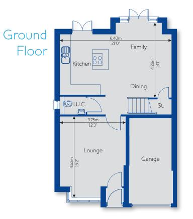
Note: All dimensions are maximum and account for alcoves, and a tolerance of  $\pm\,75\mathrm{mm}$  should be allowed.
