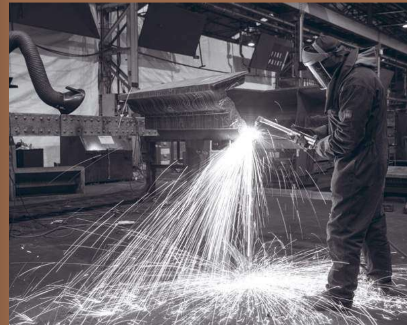
Highly skilled craftsmen in Yorkshire carefully refurbish the immense gasholder frames piece by piece
