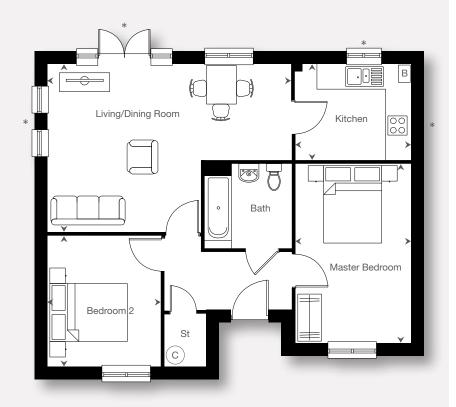
Key B - Boiler C - Hot Water Cylinder St - Store
