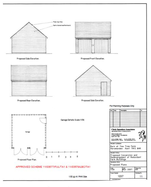
Outside there is permission for a timber framed double garage with the design complementing the agricultural style of the oast. The building will be clad in dark stained weatherboarding under a clay tile roof
